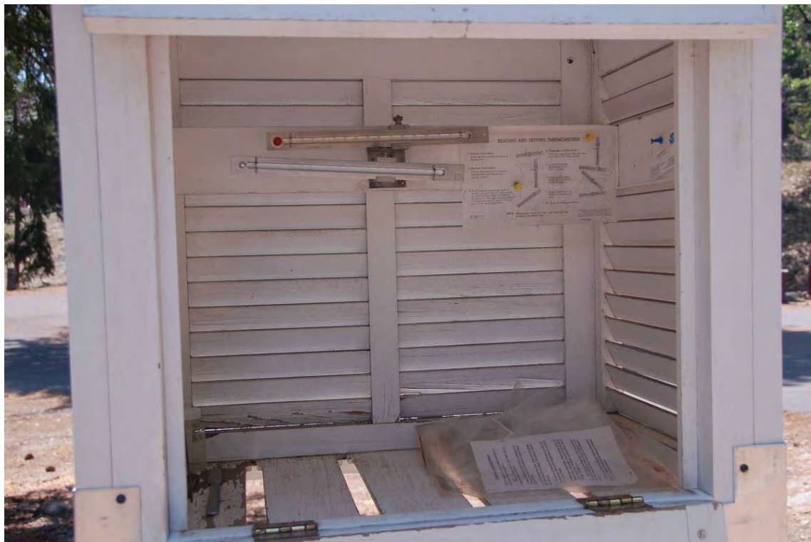
Photo 5. Cherry Valley shelter and temperature sensors
